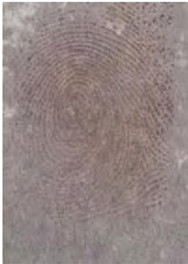
*Photo 16. Silver nitrate print after 10 minutes exposed to light. Some ridge lines are starting to appear.*
