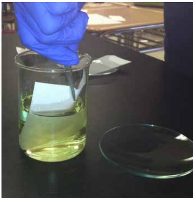
*Photo 1. Dipping the latent print left on the small paper square into the beaker*
