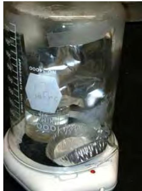
Photo 7. Superglue fuming in 1L beaker in the fume hood. The white residue is the superglue.
