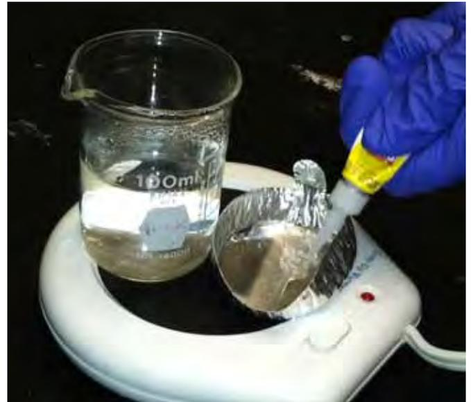
Photo 6. Hot water in beaker and metal tray with superglue on candle warmer
