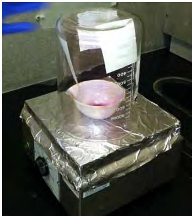
*Photo 11. Placing the beaker with the prints taped inside over the evaporating dish with iodine crystals.*
