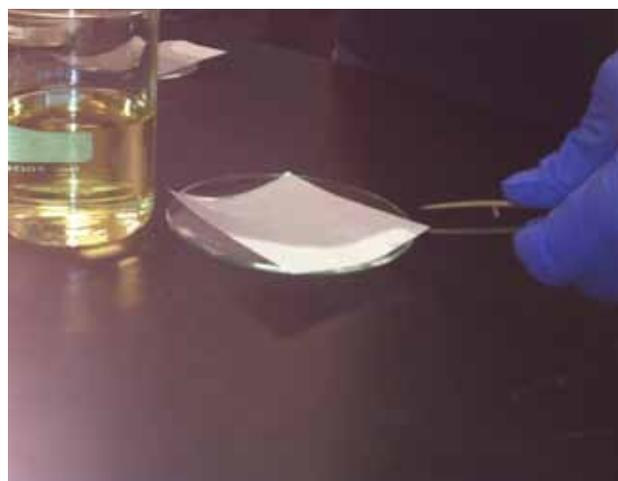
*Photo 2. Laying the print wet with ninhydrin on the watch glass to dry*
