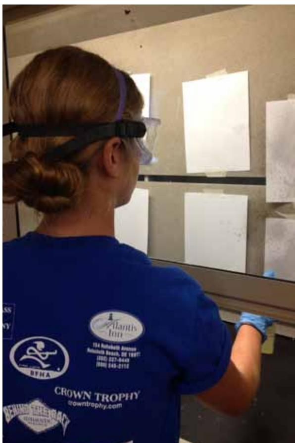
*Photo 3. Using steam over a water bath to speed up the development of ninhydrin prints*
